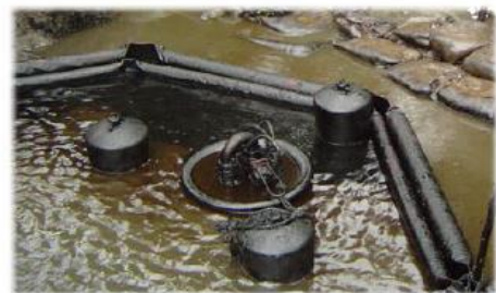
f) Pump skimmer (Source: Ro cleandesmi)
